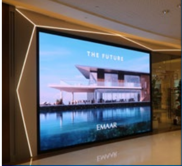
Emaar Properties Dubai, United Arab Emirates 1800 lines x 2560 columns 1.9 mm ZPN series
